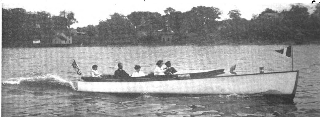
A Thirty-Foot Elco Express Launch. Engine 65-H.P. Elco. Speed 22 Miles per Hour
